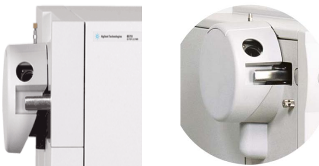
Figure 2: Agilent Technologies Electrospray Ionizer Source used for analysis by Liquid Chromatography Mass Spectrometry
