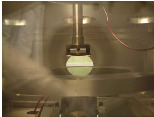
Figure 3 EHD Nozzle Inside Vacuum Process Chamber
